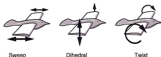
Fig. 1 Flapping motion can be decomposed into three basic motions: sweep, dihedral, and twist.
